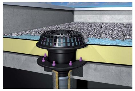
Flat roof drains made of *Ecoguss* are available in the diameters  $\emptyset$  75,  $\emptyset$  110 and  $\emptyset$  125 mm. In addition to a practical leaf trap (basket) to prevent blockages, flat roof drains are also available as an option in heated versions to allow proper function during winter.
